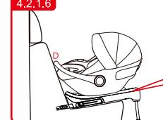
Pull the infant carrier into the base, and ensure that the handle is in its upper position D.
