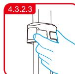
Squeeze the support leg adjusting button to retract the support leg.
