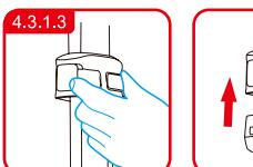
Squeeze the support leg adjusting button to retract the support leg.
