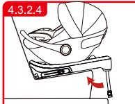
Finally, rotate the support leg and insert it into the slot at the bottom of the seat.
