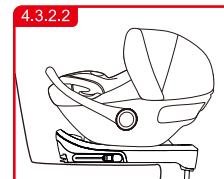
Press the ISOFIX release button to slide the ISOFIX connectors to separate the base and the seat.
